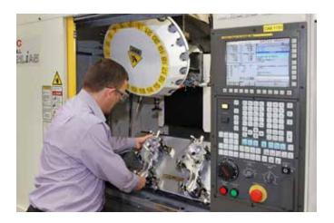
"The Robodrill was also ideally sized in terms of its tool capacity, as our applications require 20 tools and the machine's turret-type magazine houses 21 cutters." Concentric knew that the fourth axis arrangement on each machine would be critical to achieving the required TAKT times for the new oil pump and transmission pump.
